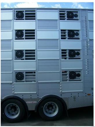
Minimum Nominal air flow requested by Reg. 1/2005/CE: 60 m3/h for each KN (100 Kg) of payload
