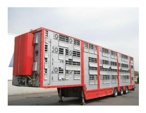
Water tank capacity = Min 1,5% of pay load
