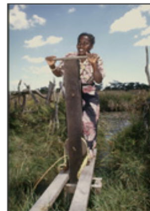
A woman works a treadle pump to irrigate crops. The Technical Cooperation Programme gives support to
